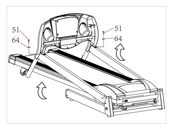
• Hold the console frame, use the 5# Allen Wrench, lock the console frame onto left and right upright tube with bolt M8\*16(51)& lock washer (64) as the picture above.
