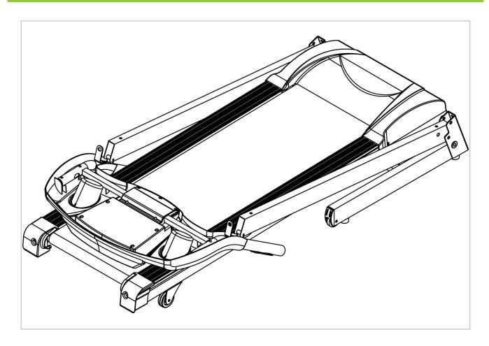
• Open the carton, get out the above spare parts, put the Main Frame on the level ground.
